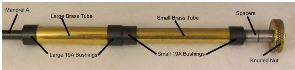
1. Assemble the blanks on the mandrel using the 19A bushings. Select the appropriate bushings for the right place. This can be done by comparing each bushing to the appropriate hardware. The 2 larger bushings are used for the cap blank and the 2 smaller ones are used for the barrel blank.
